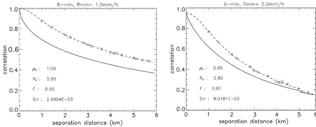
**Fig. 5.** Spatial correlation derived from one month (October 2004) of 6 min rain retrieved from radar measurements by ZPHI<sup>®</sup>. The fitted function  $\rho_A(h)$  and the associated  $\rho(h)$  are represented by the dash and the solid line, respectively. At the top (resp. bottom), only rain rates larger than 1 mm/h (resp. 5 mm/h) are considered.
