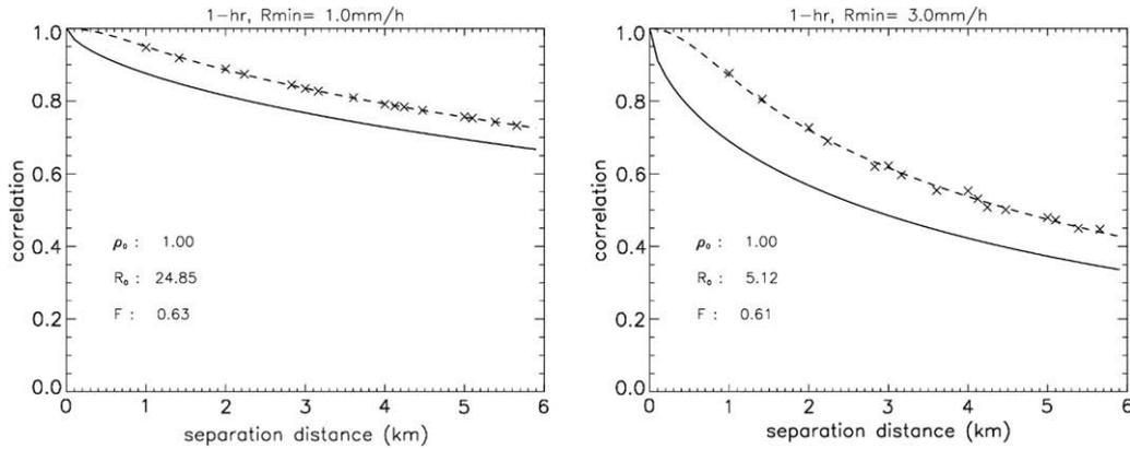
**Fig. 4.** Spatial correlation derived from one month (October 2004) of hourly rain retrieved from radar measurements by ZPHI<sup>®</sup> over the whole scan. The fitted function  $\rho_A(h)$  and the associated  $\rho(h)$  are represented by the dash and the solid line, respectively. At the top (resp. bottom), only rain rates larger than 1 mm/h (resp. 3 mm/h) are considered.
