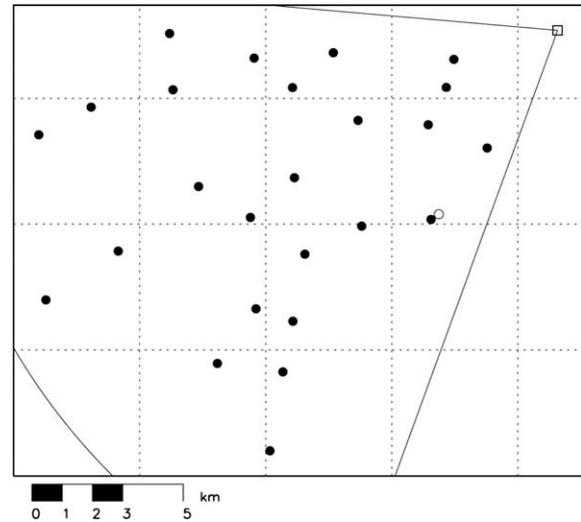
Fig. 1. layout of the rain gauge network (●), the radar (□) and the disdrometer (○). The sector covered by the radar is display (limited to 25 km range).
