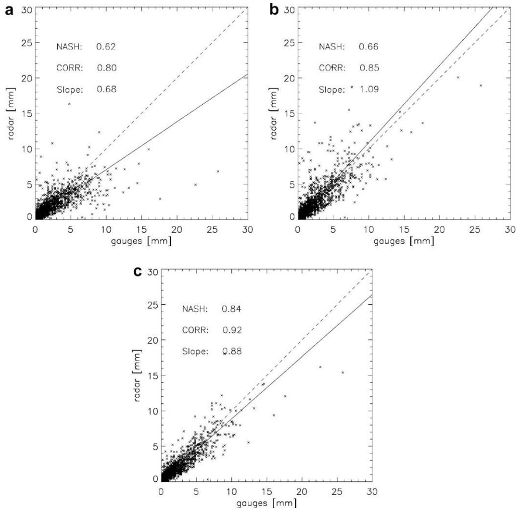
**Fig. 2.** Point by point comparison of hourly rainfall observed by the radar (vertical axis) and the rain gauges (horizontal axis) – 13 months of data October 2004–2005. The radar estimate is interpolated at the rain gauge site. (a) “Classical Z–R” estimate. Upper (b) “attenuation corrected  $Z_c$ –R” estimate. (c) Standard “ZPHI<sup>®</sup>” estimate”.
